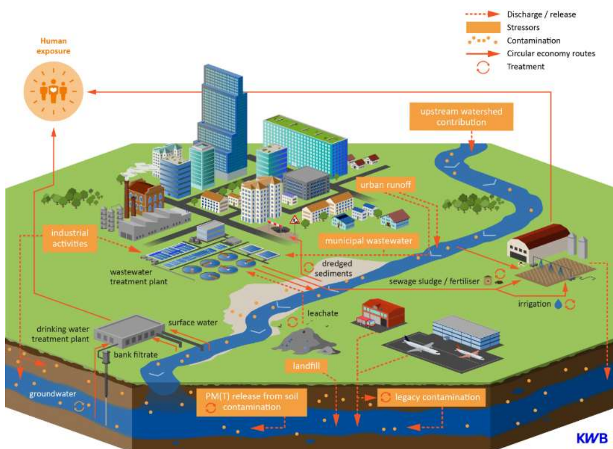
Figure 2.1 The urban water cycle and how PFAS travels through the compartments. Made by Kompetenz Zentrum Wasser Berlin (KWB) for PROMISCES.eu.
