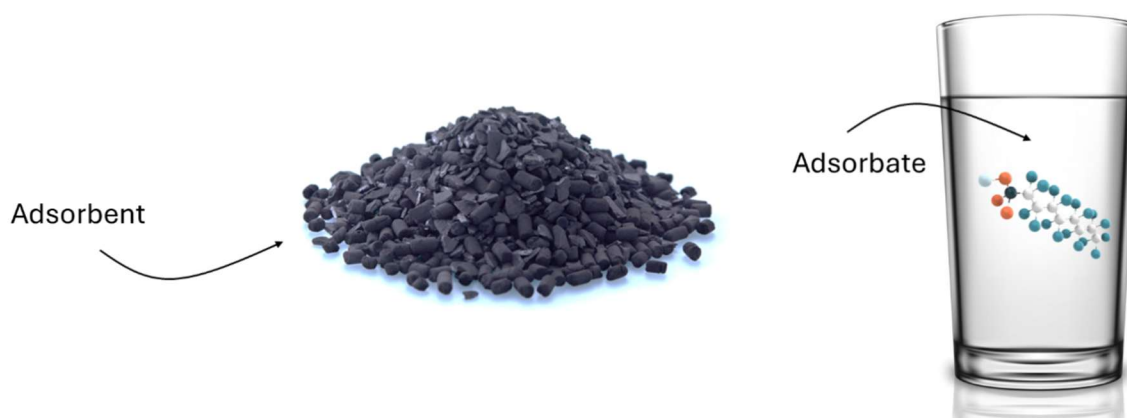
Figure 4.2 showing how the activated carbon ( adsorbent ) adsorbs the pollutant ( adsorbate ). (Figure by K.M. Lompe)
