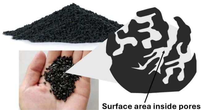
Figure 4.1 Activated carbon – a highly porous adsorbent with a large specific inner surface. (Figure by K.M. Lompe)
