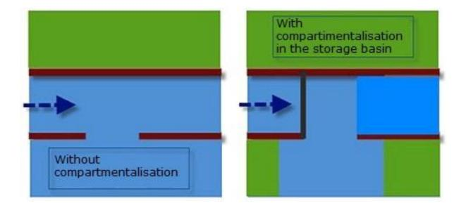
There are different types of permanent compartmentalisation structures. The Rhineland water board, for example, operates the following types: inflatable weirs, shutter weirs, stop logs, sliding structure, lift gates, floodgates and lockable culverts (Nelen & Schuurmans Consultants, 2004).
