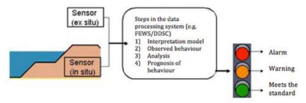
A possible tool for interpretation is data-driven modelling, which enables detection of changes in dike behaviour under similar loads. The premise is that action must be taken when abnormal dike behaviour is observed. The change in dike behaviour can be seen in fluctuating monitoring results.
