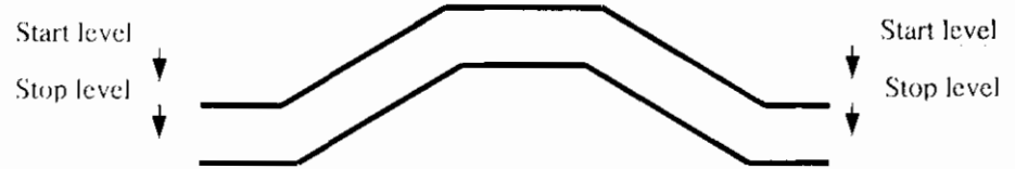
Figure 2.3 Operation levels of a siphon.
