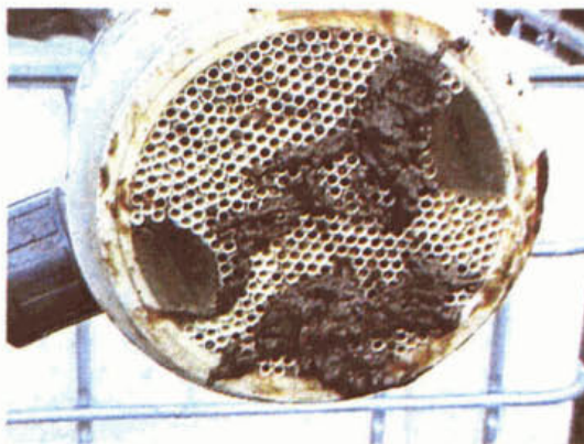
Figure 10 - Debris on the membranes
