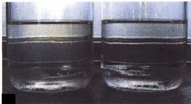
Figure 1 - WWTP effluent and MBR permeate
