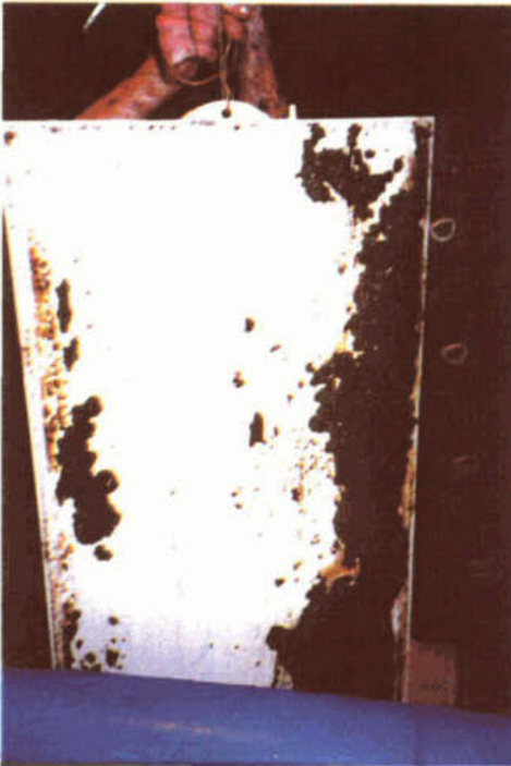
Figure 14 - Effect of a blocked aeration system
