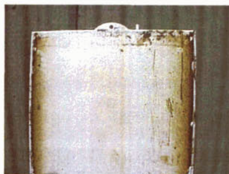
Figure 4 - Bio-fouling after software problems occurred in a Beverwijk Pilot
