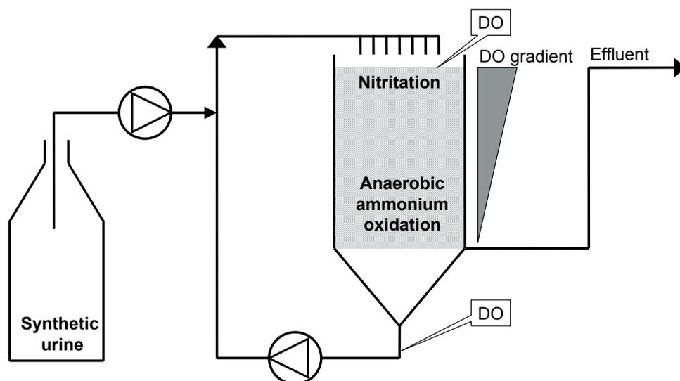
The temperature inside the reactor equalled room temperature, which normally varied between 22 and 24°C. The pH was not controlled, except at one occasion, described below. Figure 3 shows a schematic drawing of the reactor. Figure 4 shows a photograph of the reactor during the start-up phase. The column was, unlike shown in this photograph, covered in black plastic to prevent oxygenation by algae.
