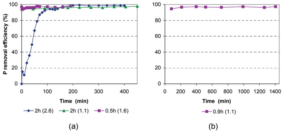
Some precipitant was always present in the effluent, reducing the total removal efficiency to around 92%. Scaling on reactor wall and the effluent pipe occurred in all experiments. Higher mixing velocity in general reduced the amount of precipitate on reactor wall and effluent pipe. However, at the same time mixing power was transferred to the settling compartment, resulting in outflow of some precipitant.
