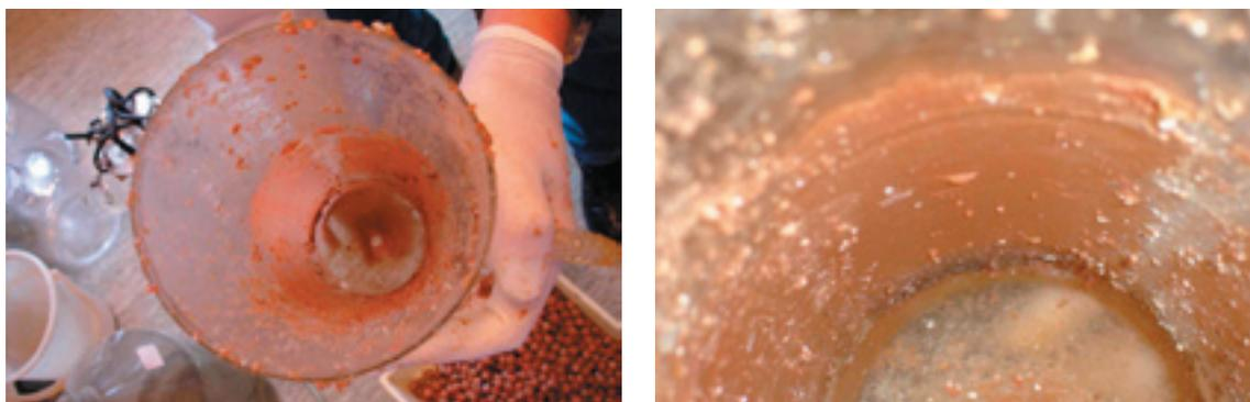
The scales were analysed with X-ray diffraction, but only amorphous states could be detected and no clear phases. Salts were most probably  $\text{CaCl}_2$  or  $\text{CaCO}_3$ . In this case, with no evidence of struvite scaling inside the reactor, struvite could best be recovered as potassium struvite after biological treatment.
