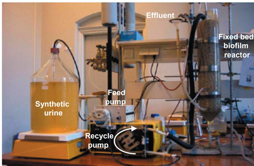
The nitrogen removal capacity of the FBBR was calculated from the sum of ammonium and nitrite removed minus nitrate produced (from anammox metabolism), based on the known influent concentrations, influent flow rate and measured effluent concentrations.
