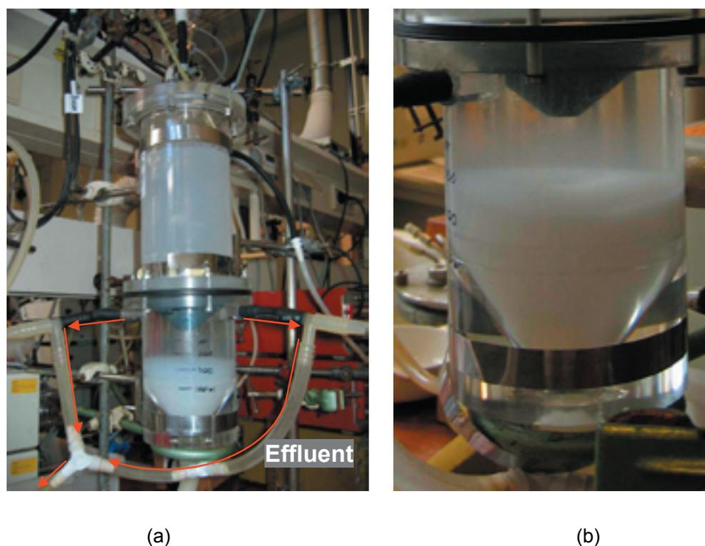
The hydraulic retention time had little or no effect on the phosphate removal efficiency above 1.6 hours, as was the case with ammonium struvite precipitation in the reactor with upright cone. Effects of mixing intensity were not investigated to the full, but it is believed that an optimum has to be found. At a too high mixing intensity, centrifugal forces move phosphate
