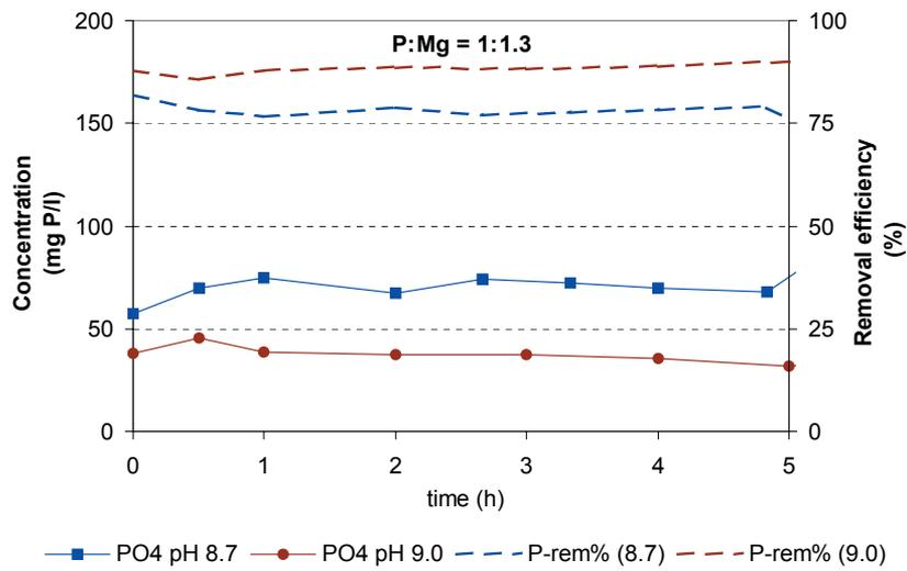
The hypothesis that lower pH ensured lower supersaturation and therefore better crystal growth seems correct, but this comes at the price of reduced phosphate removal efficiency. The difference in settling characteristics probably does not justify the lower removal efficiency. This is already a compact process and more settling space should be provided.
