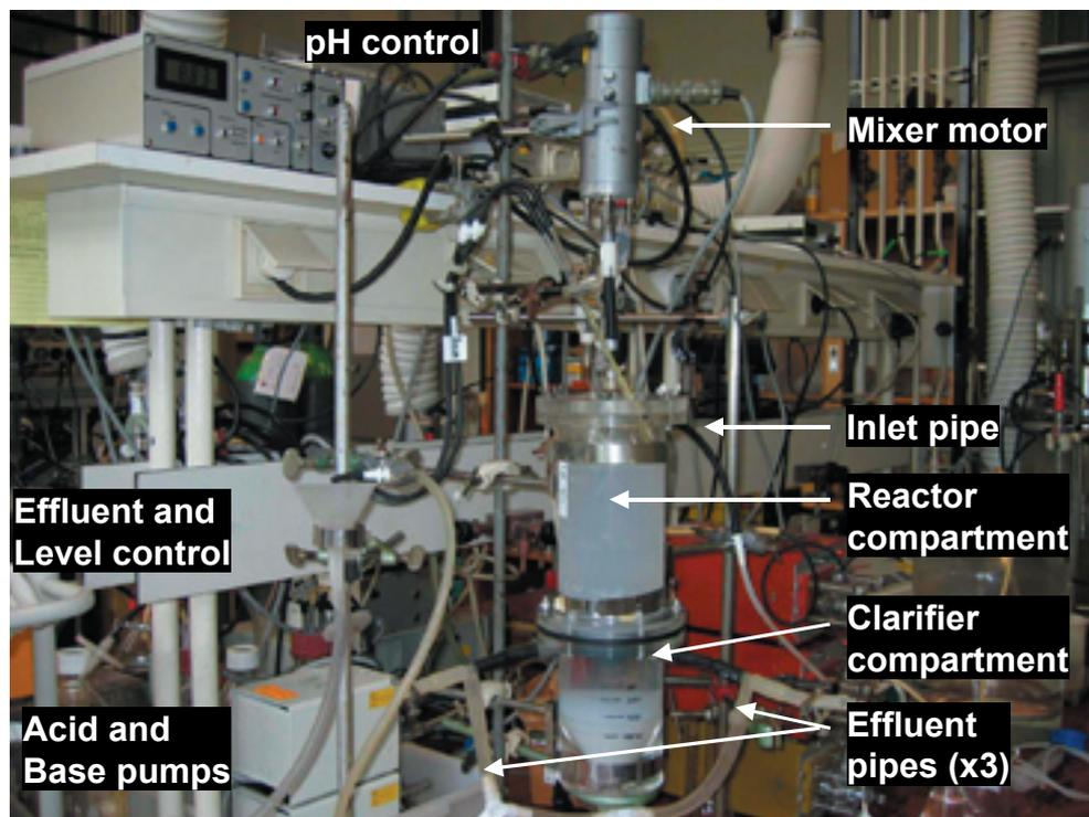
The reactor had height of 300mm and diameter of 100mm. The volumes of the precipitation section and the settling section were both 0.77l.
