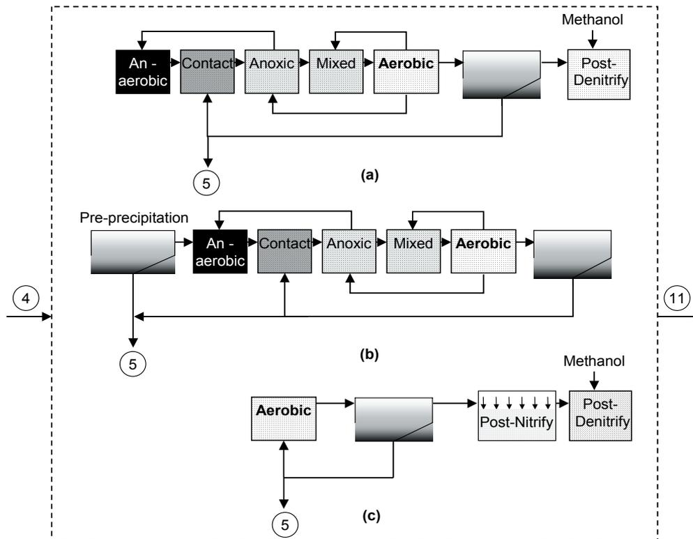
Sludge handling consists of the same unit operations for all options: Excess sludge is treated in an anaerobic digester to produce methane. In the IntWUT-BCFS process, primary sludge goes to the anaerobic digester with a smaller amount of excess sludge. We assumed dewatering by means of centrifugation. De-watered sludge is then incinerated. Liquid from the sludge dewatering normally has high ammonium and phosphate concentrations and is here mixed with urine and treated together.
