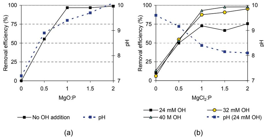
In all four cases, described above, almost all phosphate was removed at  $Mg:P = 1$ , regardless of magnesium source or whether ammonium or potassium struvite is precipitated. As with other research, a pH of 9 was crucial for precipitation and complete phosphate removal.
