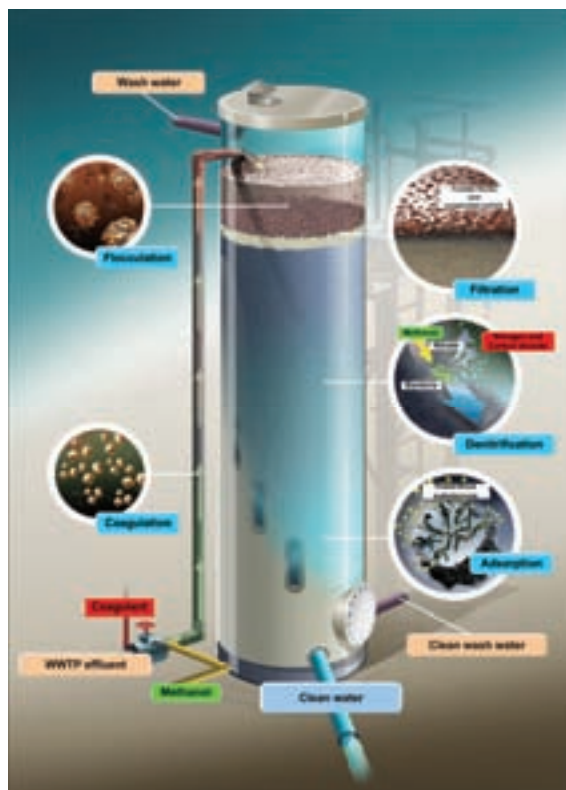
SUB-PROCESSES IN THE 1-STEP® FILTER
