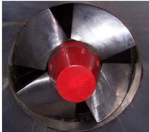
Figure 1: Kaplan turbine blades
