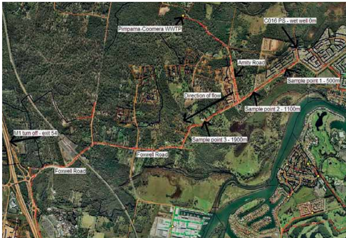
FIGURE 23 AERIAL PHOTOGRAPH OF THE C016 RISING MAIN. SAMPLES WERE COLLECTED FROM THE C016 PUMP STATION WET WELL (0 M), SAMPLE POINT 1 (AT 500M), SAMPLE POINT 2 (AT 1100M) AND SAMPLE POINT 3 (AT 1900 M)
