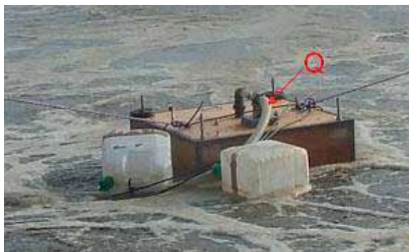
SAMPLING BOX FOR AERATED SURFACES
