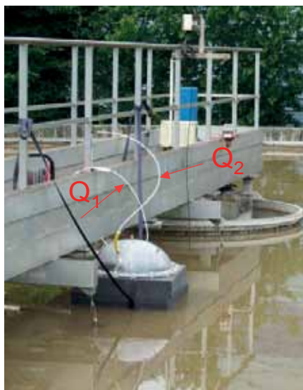
SAMPLING BOX FOR NON-AERATED SURFACES
