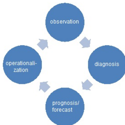
FIGURE 3.1 THE FOUR SUBPROCESSES OF THE INSPECTIONS OF FLOOD DEFENSE SYSTEMS
