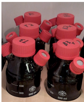
FIGURE 2 BMP BATCH REACTOR BOTTLES IN THE INCUBATOR
