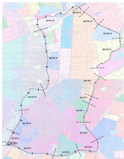
FIGURE 38 DIKE SECTIONS ALONG HEERHUGOWAARD POLDER (ARCADIS, 2011)
