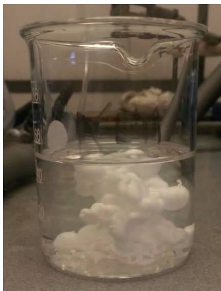
EXAMPLE OF POLYMER PRECIPITATE IN ACETONE
