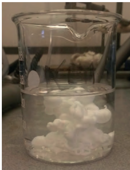
EXAMPLE OF POLYMER PRECIPITATE IN ACETONE
