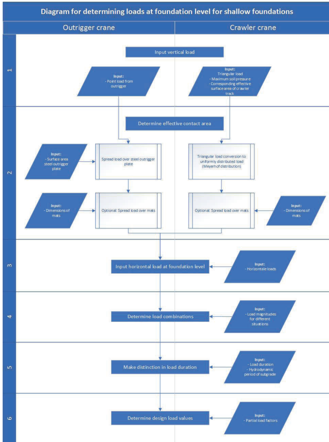
FIGURE 5-1 DIAGRAM FOR DETERMINING LOADS AT THE FOUNDATION LEVEL OF A CRANE HARDSTAND
