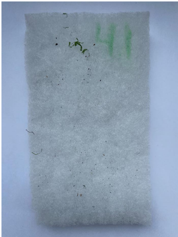
Figuur 27 Hockeykunstgras filter 4.1 microplastics score 1
