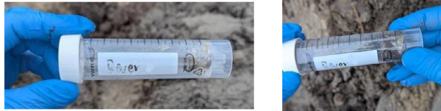
Figure 1 – Sample preparation: first, the fur was removed from the tubes (left picture) and later added of moist sandy soil (right picture).
