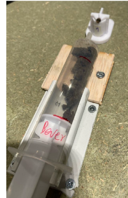
Figure 3 – Odour delivery setup. A 20 mL syringe containing the sample is placed at 2 cm from the honeybee and used to deliver the sample volatiles.
