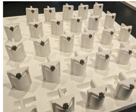
Figure 2 – Our Dr. Bug honeybees resting in 3D-printed harnesses prior to the experiment.
