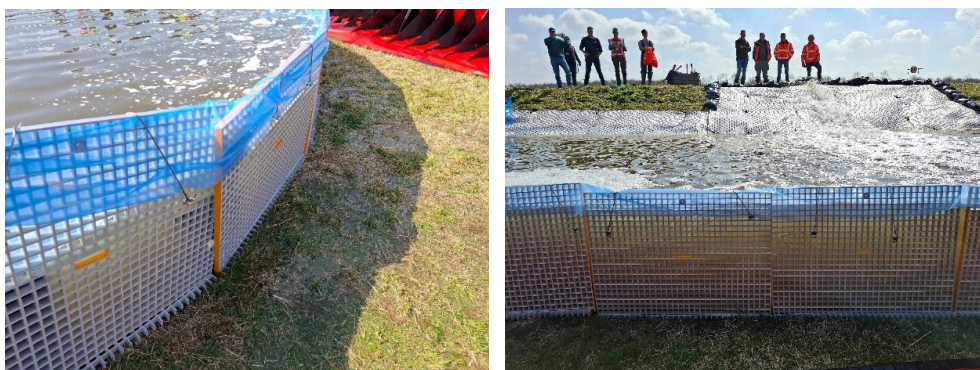
Figure 2.62 The barrier has been filled to its upper edge, and overtopping has commenced.
