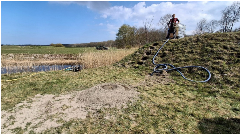
Figure 4.4 To simulate the appearance of a sand boil transporting sediment, water from a reservoir is conveyed underground through a hose to the centre of a sand-filled crater.
