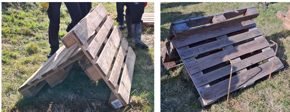
Two-pallet configuration. The pallets are anchored on the landward side (i.e. non-water-retaining side) using steel pins to prevent movement of the structure.
