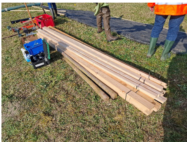
Figure 3.1 Timber battens (25 mm × 45 mm × 5 m)
