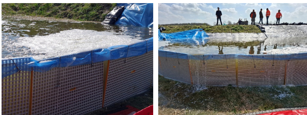
Figure 2.62 The barrier has been filled to its upper edge, and overtopping has commenced.
