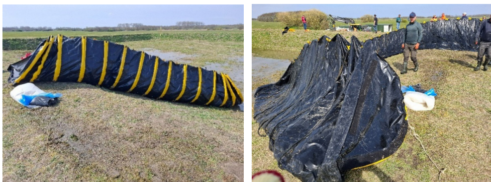
Figure 2.47 Complete removal of the residual water was achieved by turning the TubeBarrier upside down and placing it on a slope, allowing the remaining water to drain from the system.
