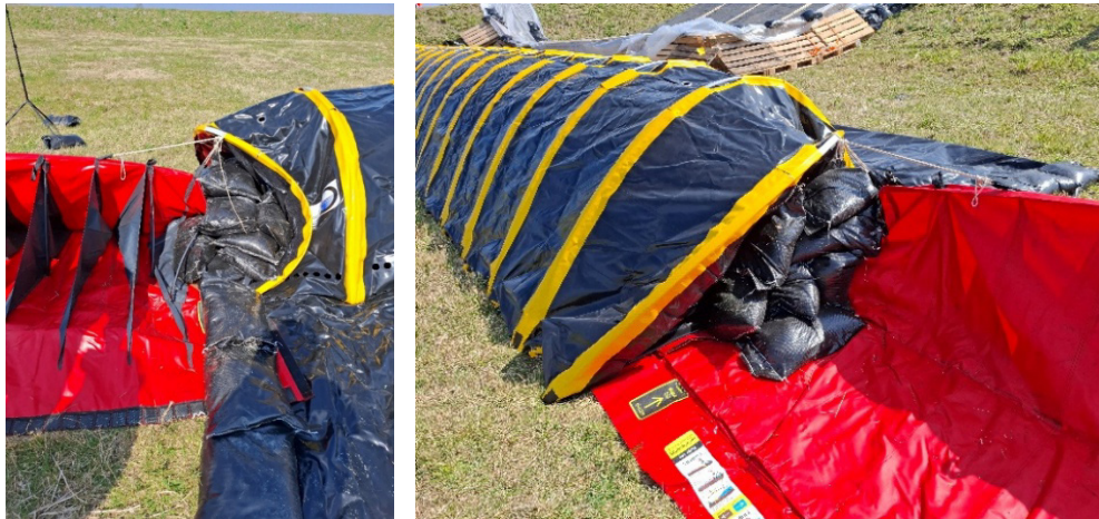
Figure 2.78 Close-up view of the connection between the BFW system and the TubeBarrier. Left: water side; right: protected side.
