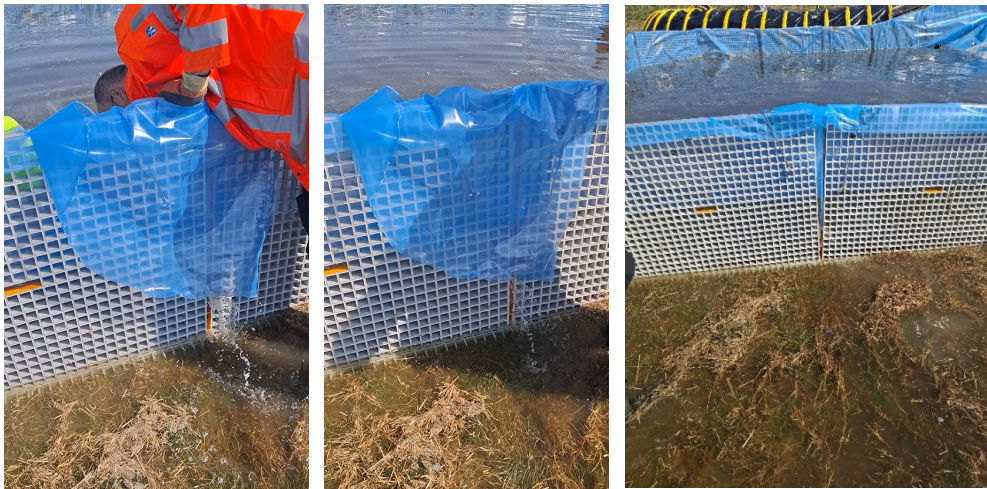
Figure 2.72 The tear was mitigated by positioning an additional membrane sheet against the two vertical panels on the water side of the barrier. This intervention resulted in a significant reduction in leakage.
