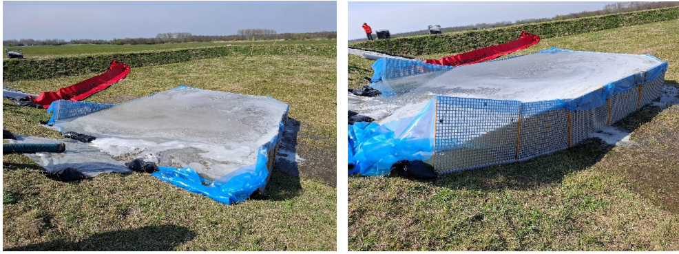
Figure 2.68 Following cessation of the water inflow, the system was able to maintain the retained water level for a considerable period. The Haawal system proved to be highly shape-stable under load. No adverse effects were observed at locations where adjacent panels were not perfectly aligned and visible gaps were present between modules.
