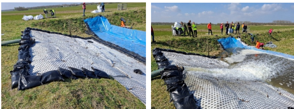
Figure 3.17 Performance testing of the Tensar geogrid reinforcement system subjected to overtopping flow.
