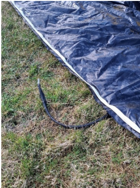
Figure 2.38 During repositioning of the TubeBarrier, a drainage pipe on the underside of the system was inadvertently pulled out, indicating the vulnerability of this component during handling.
