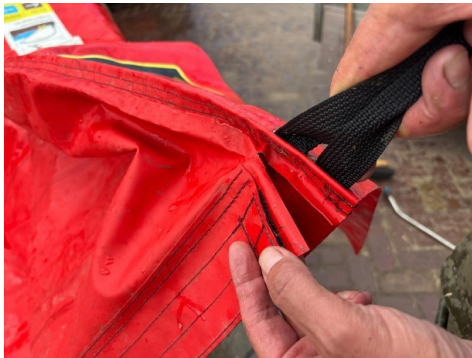
Figure 2.88 Inspection after the exercise revealed that one of the seams had ruptured during use.
