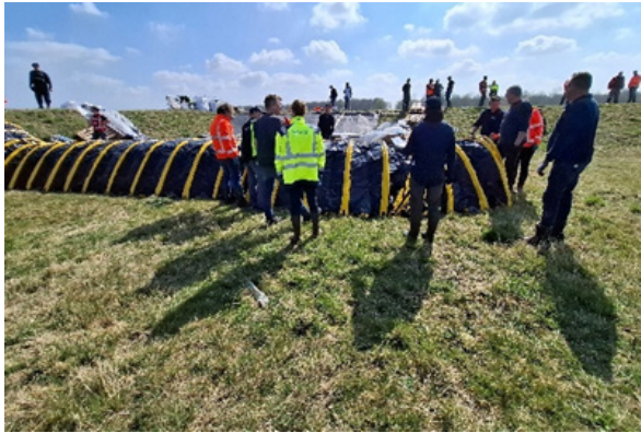
Figure 2.38 During repositioning of the TubeBarrier, a drainage pipe on the underside of the system was inadvertently pulled out, indicating the vulnerability of this component during handling.
