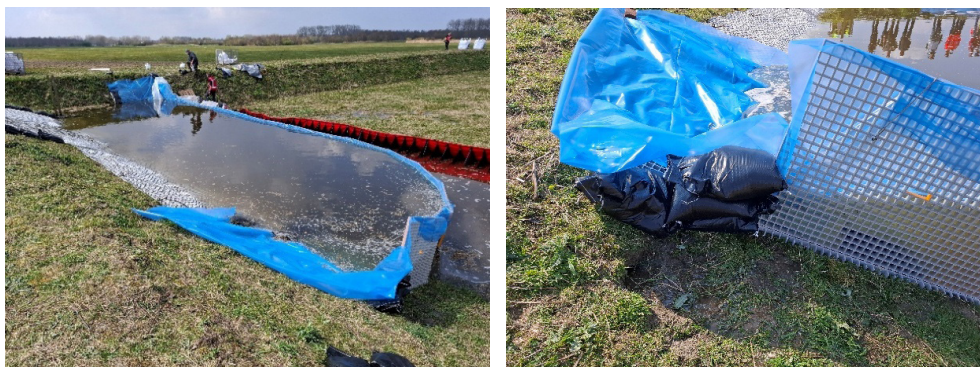
Figure 2.63 Following cessation of the inflow, the water level in the Haawal basin gradually decreases as the basin drains.
