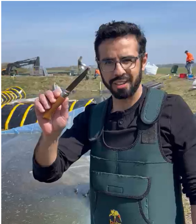
Figure 2.69 As part of the test, a volunteer wearing chest waders used a knife to create a long tear in the membrane at a location where a gap was present in the Haawal barrier.
