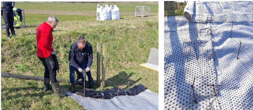
Figure 3.17 Performance testing of the Tensar geogrid reinforcement system subjected to overtopping flow.
