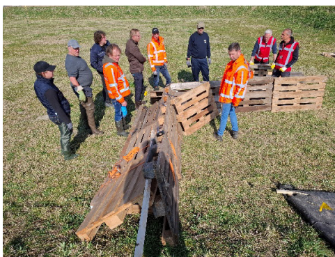
Figure 2.16 An L-shaped configuration of three-pallet modules. The corner is reinforced using an additional pallet fixed in place with metal clamps.
