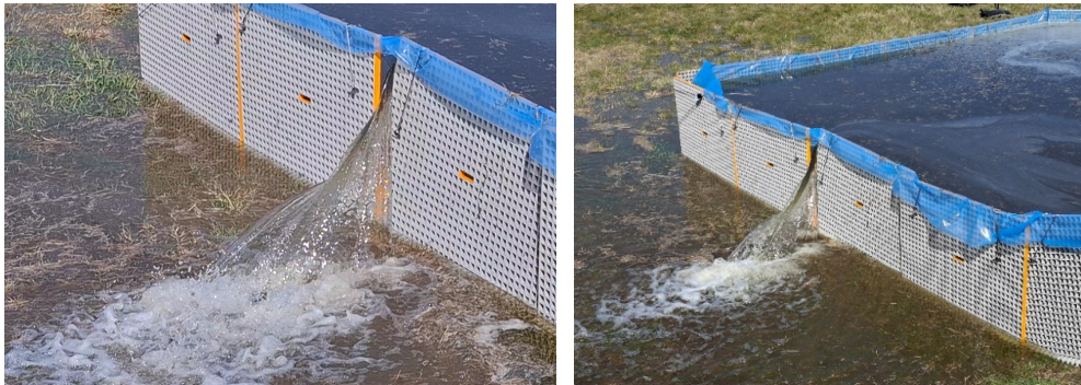
Figure 2.72 The tear was mitigated by positioning an additional membrane sheet against the two vertical panels on the water side of the barrier. This intervention resulted in a significant reduction in leakage.
