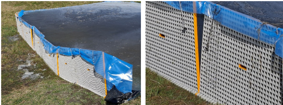
Figure 2.68 Following cessation of the water inflow, the system was able to maintain the retained water level for a considerable period. The Haawal system proved to be highly shape-stable under load. No adverse effects were observed at locations where adjacent panels were not perfectly aligned and visible gaps were present between modules.
