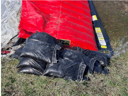
Figure 2.83 Underseepage is also observed in this configuration. In addition, part of the flow bypasses the barrier along the edges, notwithstanding the sandbag sealing applied at these locations.
