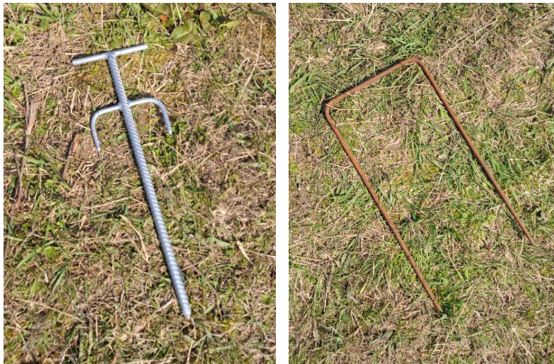
Figure 3.6 Left: steel T-pins with an additional U-shaped staple. Right: U-shaped staple (10 cm wide, 30 cm long, 8 mm diameter).
