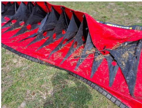
Figure 2.85 Although the grass had been cut approximately three weeks before the exercise, a considerable amount of vegetation became trapped in the BFW system during deployment. The subsequent cleaning of the system was found to be very labour-intensive.
